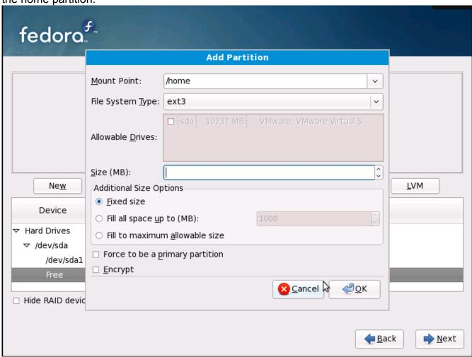
Fedora I believe requires 2.5 GB at a minimum for / (root) I fedora. F. **Add Partition** Mount Point: File System Type: ext3 Allowable Drives: Size (MB): Ne<u>w</u> LVM Additional Size Options • Fixed size Device ○ Fill all space up to (MB): → Hard Drives O Fill to maximum allowable size ✓ Force to be a primary partition
